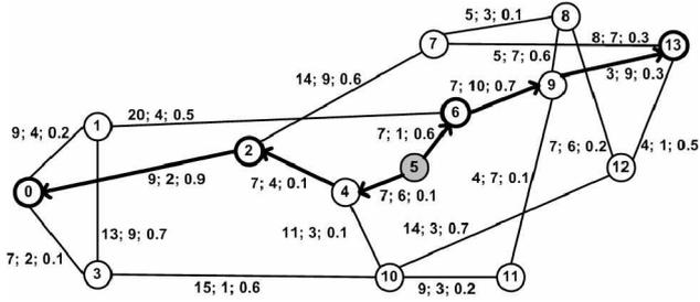
**Figure 1: The NSF Net.**  $d_{ij}$ ,  $c_{ij}$  and  $t_{ij}$  are shown over each link. Objective Functions are  $\alpha(T)=0.73$ ,  $C(T)=6.4$ ,  $DA(T)=16.5$ ,  $DM(T)=23$ . Multicast group:  $s=5$  &  $N_r=\{0,2,6,13\}$ .
