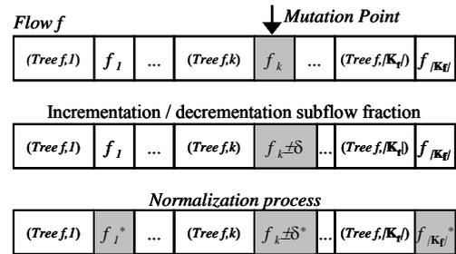
**Figure 6. Subflow fraction mutation following by normalization process.**
